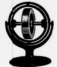
his mysterious wheel is a gyroscope. Wien set in motion, it constantly maintains a fixed position in space ... pointing straint as an arrow in whatever direction it is et.
