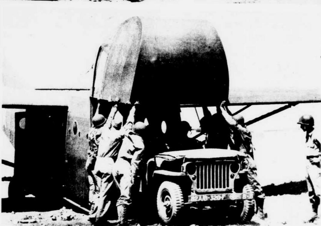
Jeeps also ride in gliders—to speed the movement of airborne troops once they have landed on enemy ground. Here's how the glider "opens wide" to let the jeep out.
