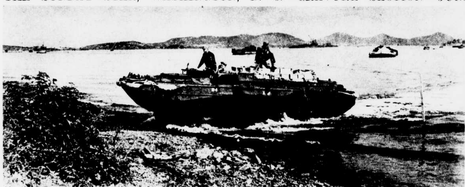
Reaching shore, the "duck" switches off its propeller and keeps rolling right up on the beach, powered by its six-wheel drive.
