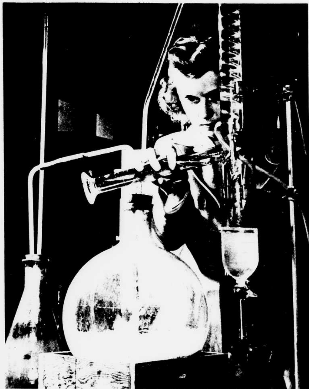
Under full production, a staff of 100 chemists and analysts will keep a close check on all processes in the plant laboratories. Here Lauralene Orr, 22, tests synthetic rubber latex for impurities.
