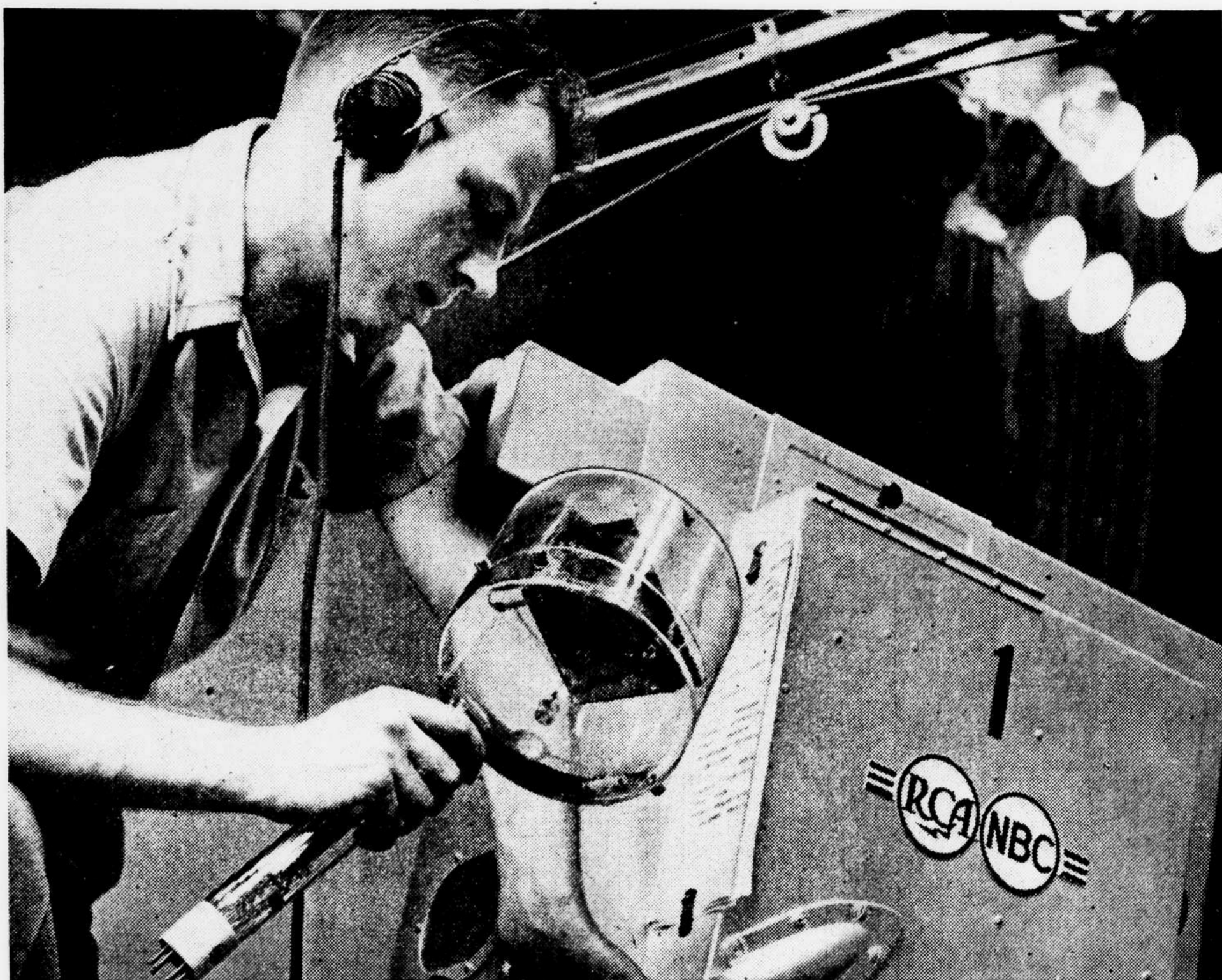
Here, an NBC technician is installing an Iconoscope—the RCA invention that made possible electronic television.
