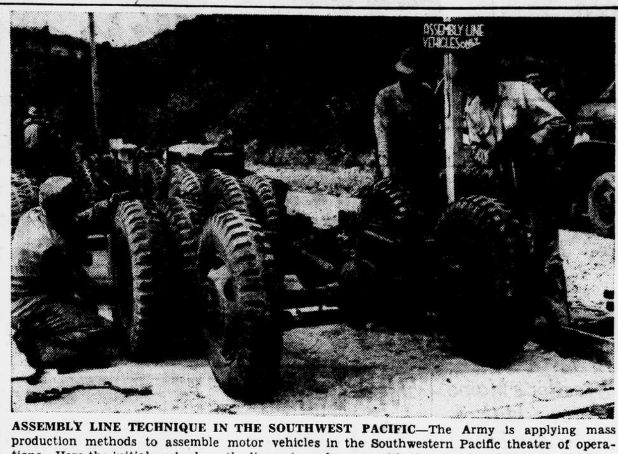
ASSEMBLY LINE TECHNIQUE IN THE SOUTHWEST PACIFIC—The Army is applying mass production methods to assemble motor vehicles in the Southwestern Pacific theater of operations. Here the initial push along the line gets under way with the rear running gear
