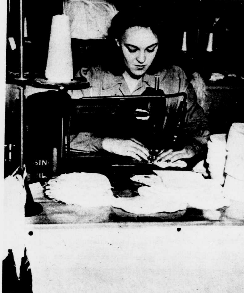
For the primer cap, at the breech end of the powder bag, the new silk fabric from the old stockings is cut into the circles which this ordnance plant worker is stitching. Fifteen pairs of silk stockings provide sufficient cloth for an average size powder bag.
