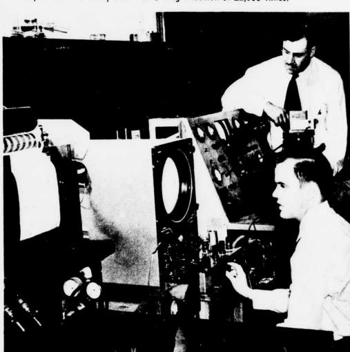
A different instrument is this scanning electron microscope, another RCA development, which makes a picture of metal surfaces in detail never before possible. It employs the principles of television and radio facsimile, in conjunction with electron microscopy, to build up a picture by minute elements of different intensity. It "sees" particles as small as a 500,000th of an inch.
