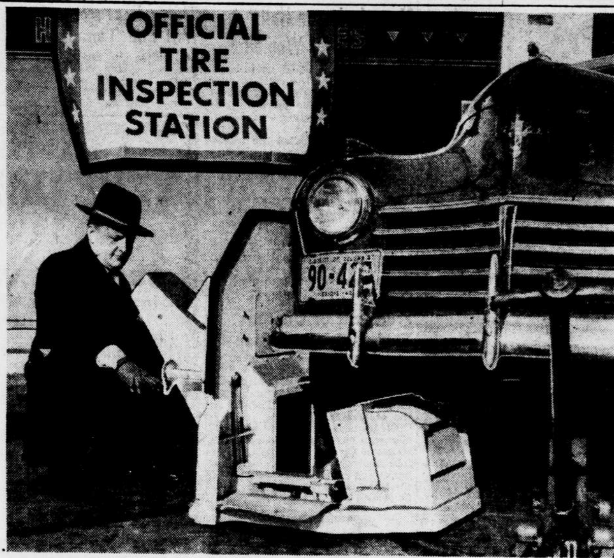
ANY TACKS OR CRACKS IN YOUR TIRES? —These two pictures present a preview of scenes which will begin all over Washington as District motorists start visiting tire inspection stations Tuesday. A novel X-ray machine is shown above, being operated by C. L. Powell, manager at the Firestone station at Thirteenth and K streets N.W. This outfit found a long piece of screw-driver embedded in a tire casing the other day.
