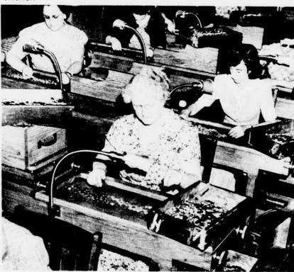
Here the blank nickels are inspected for defects before they go to the stamping machine. Bad ones go back to the smelter.
