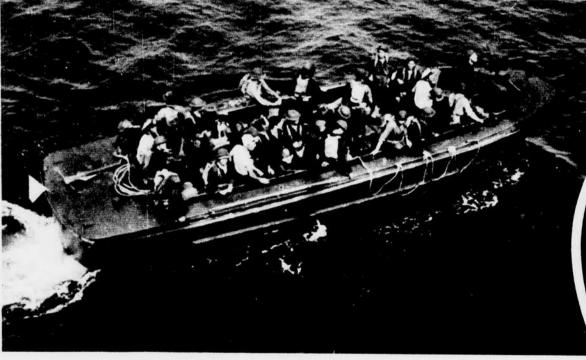
Close-up of a landing barge heading for shore with its load of troops. Note machine gun on bow and armored pits for gunners.
