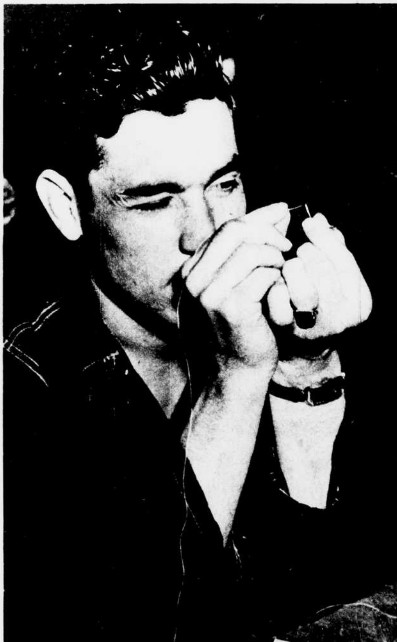
Sharpening his needle eye. Technician Fifth Class Joseph McCafferty threads one of the curved needles used in the important job of sewing up rips and patching the balloon fabric.
