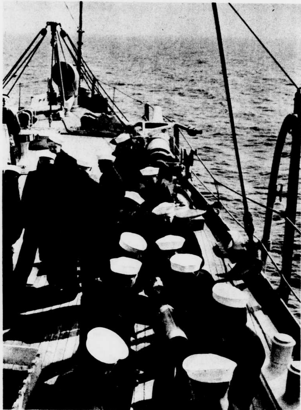
In its metal casing a 4-inch shell is passed up from below along a double line to a waiting gun. The casing protects the shell from corrosion.
