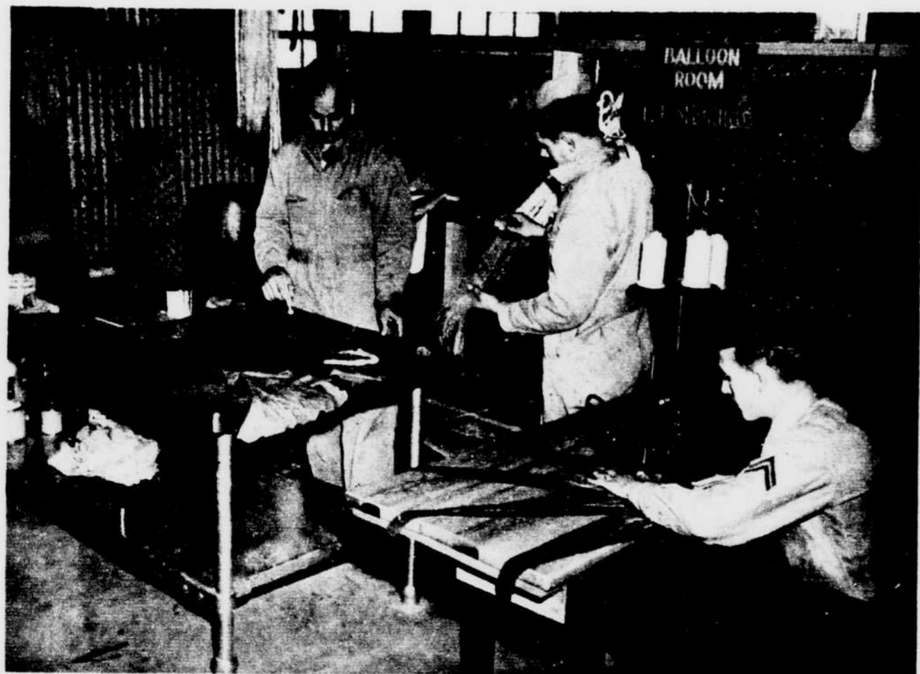
In the barrage balloon shop marines learn how to repair the giant bags. The corporal at the sewing machine is making a "finger patch." Man in the center is learning how to braid hemp. A. P. and Wide World Photos.
