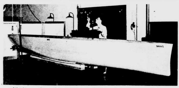
Weighing a ship model preparatory to ballasting it to the proper displacement, draft and trim.
