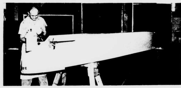
Installing model propellors on a model for self-propulsion test in the basin. The standard model length is 20 feet.
