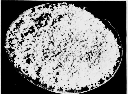
Here are milk curds washed and dried into the ricelike substance that is dried casein. After this casein is ground and treated it is ready for the fiber factory.
