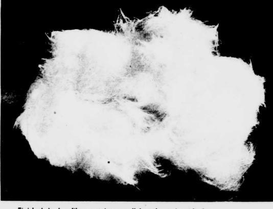
Finished Aralac fiber, cut into small lengths and ready for blending with other textile fibers. It can be cut into any lengthfrom half inch to a half mile.
