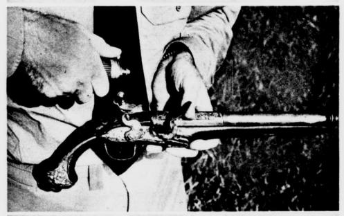
After loading pellet and powder through the muzzle, the flash pan is primed with fine powder.
