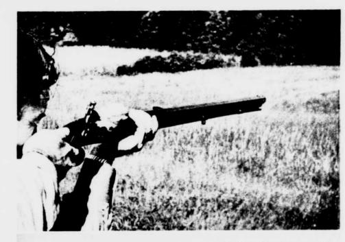
This movie series shows the firing of an English flint-lock sporting rifle. The gun is .56 caliber with rifled bore, shooting conical bullets. It was made about 1820 by Barnett of London. Here the flash in the pan is just starting
