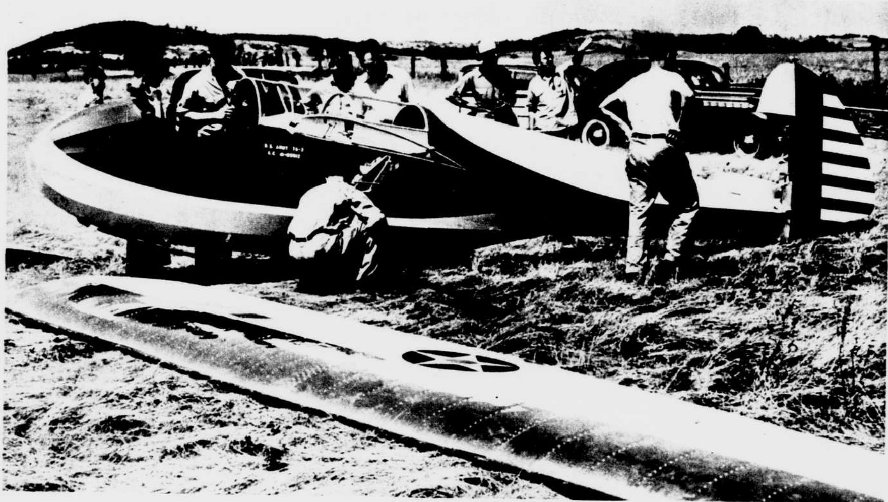
Assembling the first glider for the Army Air Corps at Elmira. At this stage the wings, one of them seen on the ground, are about to be attached to the body of the glider.
