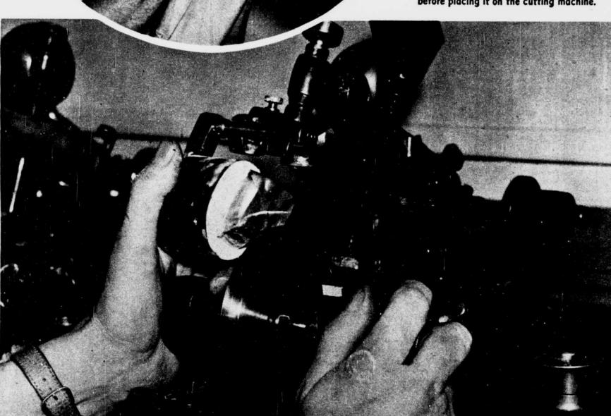
Closeup of the stone on the cutting machine. Diamond dust is mixed with olive oil on the paper-thin cutting wheel. Actually it does not saw, but polishes the cut deeper and deeper." Wide World Photos.
