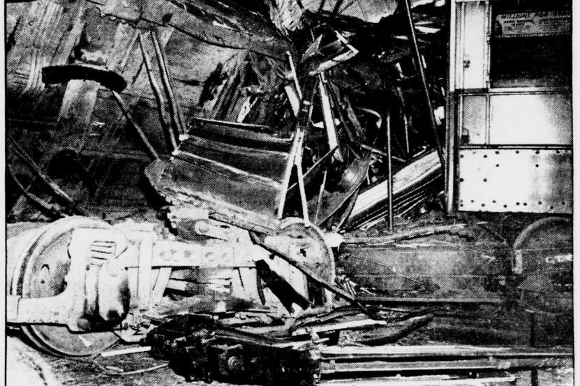
A close-up of the wreckage, indicating how the striking car ploughed into the middle of the other, forcing passengers of the northbound car to kick their way through windows to make an
