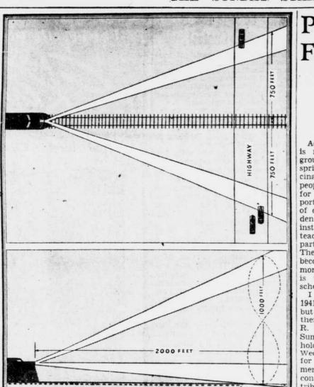
This drawing shows how safety light works on Southern Railway's new streamliners going into service this month.
