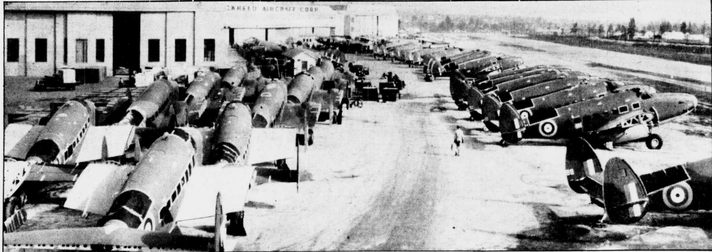
BURBANK, CALIF.—BOMBERS FOR BRITAIN FLOW FROM LOCKHEED PLANT—Production of Lockheed Hudson bombers for Britain has been so accelerated recently that final assembly of the planes is being done outdoors on airports near the plant. Here are several score of camouflaged ships waiting for installation of wing tips and motors on the airport adjacent to the plant. —A. P. Wirephoto.
