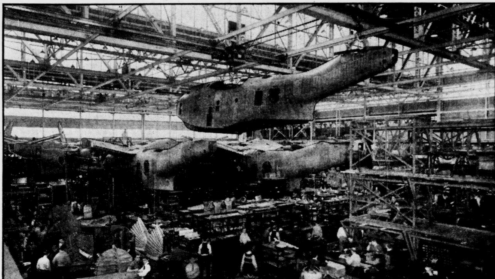
BALTIMORE.—WITH THE GREATEST OF EASE—A Navy air levathan soars aloft, without wings, in the Navy Bay of the Glenn L. Martin Co. The hull of the 20-ton PBM-1 patrol bomber, destined to join the long-range guardianship of our coasts, is swung by a power crane 40 feet above the Nation's largest aircraft assembly floor. Thus emerging from the steel hull fixture, it will receive its beaching gear and roll forward
