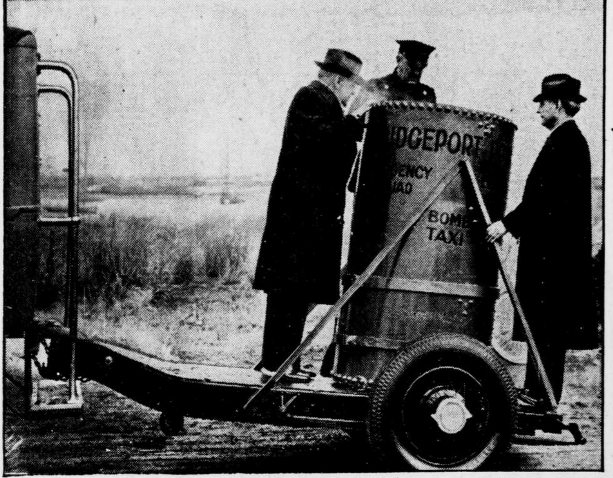
CAPITAL MAY GET ONE OF THESE "BOMB-BUSTERS"—This homemade contrivance for carting off suspected bombs in safety has caught the eye of Police Chief Ernest W. Brown, who hopes to order one for his own force. It is the invention of police at Bridgeport, Conn., and was improvised from an old locomotive boiler and an automobile chassis.
