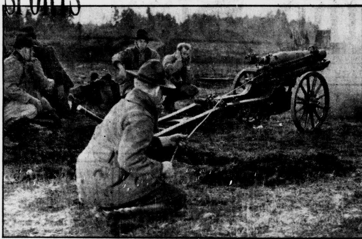
FORT LEWIS, WASH.—ARMY TRIES OUT PACK HOWITZERS—Using live ammunition, Battery C of the 90th Field Artillery tried out this new 75-mm. pack howitzer in practice firing recently. The soldier in center foreground has just pulled the firing cord while a soldier (background) holds his ears. The gun, designed for transportation by mule pack, is the first of its type received at the fort.
